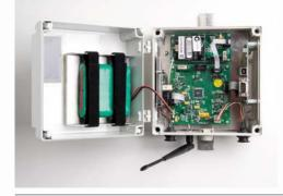
Developed from Data Node technology, the Radio Node is a data storage unit that uses ISM 900MHz radio to routinely transmit data to a receiving device. The data is automatically sent to either a 'Radio Receiver' or 'Network Gateway' device, where it is automatically uploaded to a PC and viewed using the included AquaSpy Display software.
