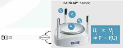
The precipitation sensor detects the impact of individual raindrops. The voltage signals U resulting from the impacts are proportional to the volume of the drops V and therefore, the signal of each drop can be directly converted to accumulated precipitation P.
