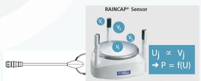
IOP vThe precipitation sensor detects the impact of individual raindrops. The voltage signals U, resulting from the impacts are proportional to the volume of the drops V<sub>j</sub> and therefore, the signal of each drop can be directly converted to accumulated precipitation P.
